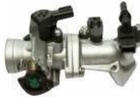
Throttle & intake tube assembly
