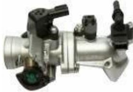
It is composed of intake pipe, TPS, idle filling valve and air-filling valve hose. The role of idle filling valve provides different intake quantities for ECU to control cold start and maintain idle speed; TPS functions to provide suitable additional fuel injection volume for emergency fuel Gates while achieving full-load fuel injection control; Throttle function provides the driver with a controlled intake of air to control the engine load.
