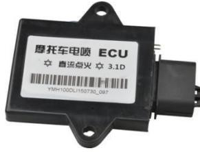
The control and management system of the electric jet system is the core part of the entire electric jet. The signals of various sensors (throttle position, engine temperature, intake pressure, speed, crankshaft position, etc.) are used as input signals, and after calculation and comparison, Determine the output signal (e.g. time of injection, pulse width of injection, filling time and ignition time).
