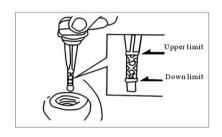
Using the recommended type of oil SAE 10W-30(SIGMA) for 4-stroke engines or its substitute HQB-10 should be used.
