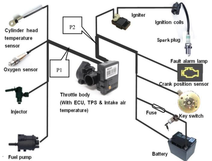
Figure I. EFI system configuration diagram
