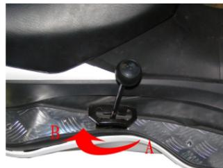
Pull from A to B for reversing gear.
