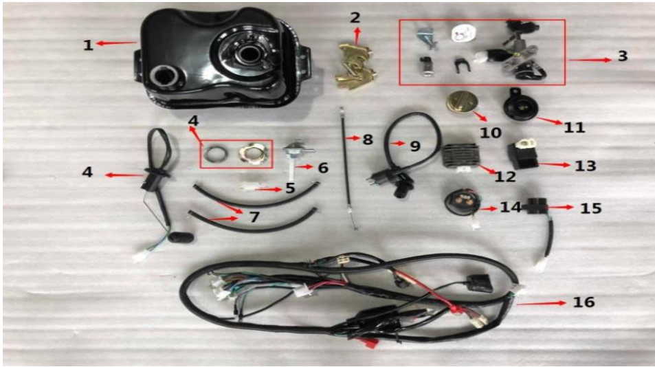
Figure: H:fuel tank, igniter, etc(图H: 油箱、点火器等)
