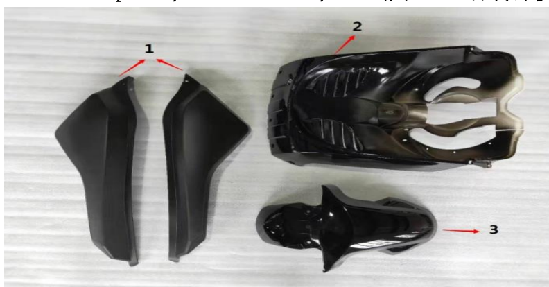
Figure K: (decorative plate, front fender, etc (图K: 左右装饰板、前泥板等))
