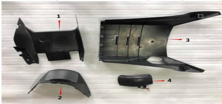
Figure J: fuel tank bottom, Glove box front cover, etc (图J: 油箱底板、杂物箱前罩)
