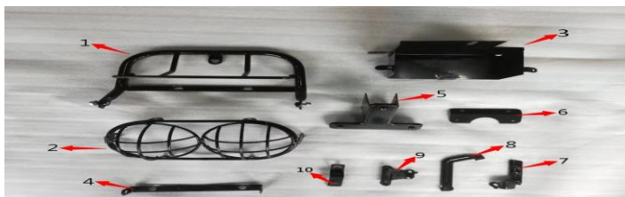
Figure G: headlight bracket, headlight cover, etc (图G: 大灯支架, 大灯网罩等)
