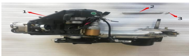
Figure N: engine, axle, nut (图N: 发动机、发动机轴、螺母)
