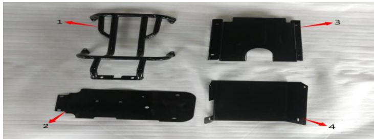
Figure M: fuel tank bracket, cover under seat, etc (图M: 脚踏支架, 坐垫下护板等)
