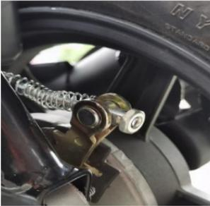
Brake adjusting Nut cap
